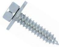
Screw, DIN 7976-compliant with captive washer, galvanised steel, blue passivated (A2K), shape C, pointed tip
