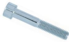
ISO 4762/DIN 912, steel 8.8, galvanised, blue passivated (A2K)
